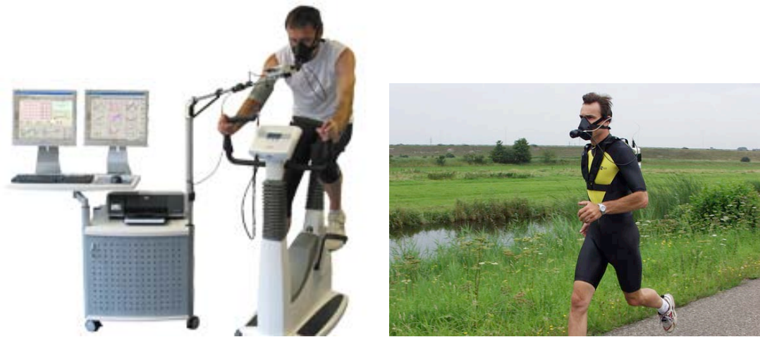
Fig. 2 On the left, a complete system for indirect calorimetry. On the right, same system but portable
